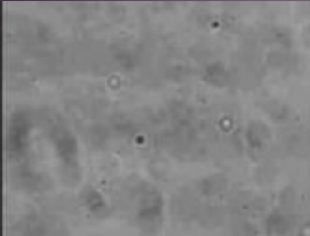
Trapped polystyrene bead using two CARS beams
