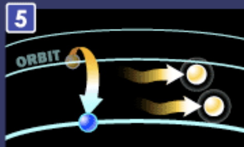
5 ...produces two photons of the same wavelength and phase.
