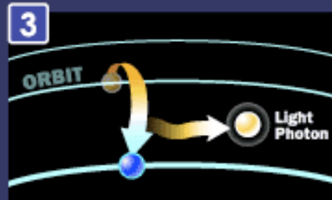
3 Electron relaxes to a lower energy state and releases a photon.
