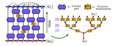
Figure 1: A spacetime diagram for a "monitored" quantum circuit, consisting of a brickwork structure of two-site unitary gates interspersed with local projective measurements. A pure-state trajectory corresponding to a particular sequence of measurement outcomes is shown, though the inherently probabilistic nature of the measurement outcomes could yield other trajectories.
